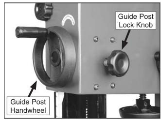
Figure 36. Guide post controls.
